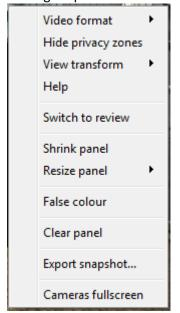
**Video format:** Allows the user to select which of the camera's video streams (which format/resolution) they wish to view.
