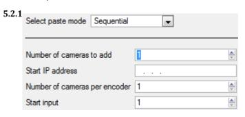
**Start IP Address** will determine the IP address of the first new camera being added. The IP addresses will be incremented from here. (So, make sure no IP addresses in this range have been used.)
