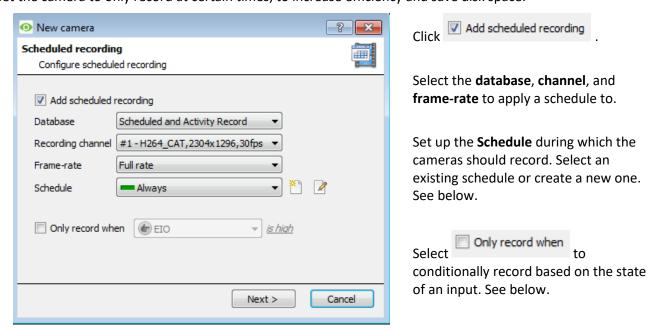
**Input Condition**: Check the box to **only record when...** then select an input from the dropdown menu, and modify the condition requirement of that input by clicking on the blue hyperlink next to the menu.
