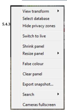
**View transform:** Allows transforming images for cameras with special lenses. (E.g. 360-degree cameras.)
