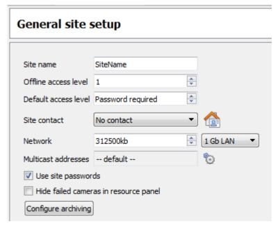
From the general setup, set the site name, default access levels, site contacts, network speed, and operator archiving profiles.
